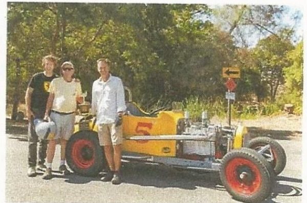
Car # 5, Class SP-2, 8.069 ET, Class SP-2, 1915 Ford Model T roadster, "B" block with a Steve Serr Miller head, '39 trans, Kiwi quick change, Model A chassis. Don Krout, Groveland, CA (L to R --- Mason, Don, Andy)
