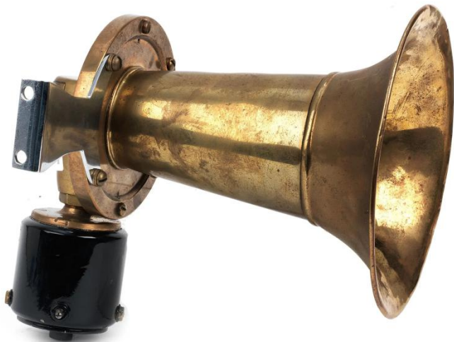
An electric car horn manufactured by Lovell-McConnell Manufacturing Company.
